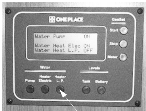
Propane Gas Water Heater Switch (Located on OnePlace® monitor panel)
