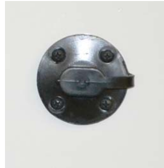
Single Solar Port (Located on an exterior sidewall or inside an exterior compartment, depending on model)
