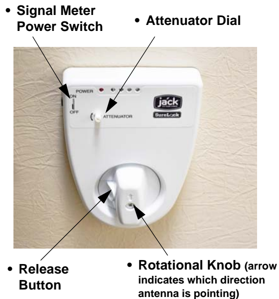
Digital Antenna Signal Meter (Located on ceiling)
