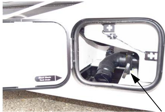
Black Waste Tank Drain Valve (Located in driver side compartment ahead of rear wheel)
