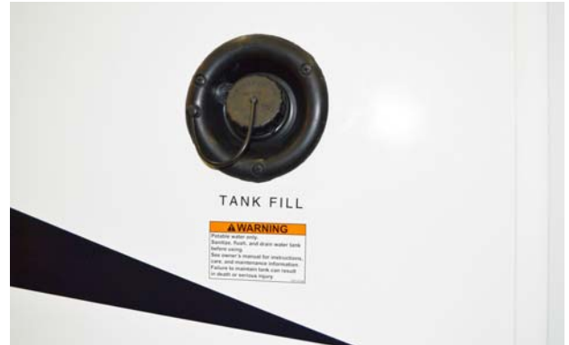
Water Tank Gravity Fill -Typical View
