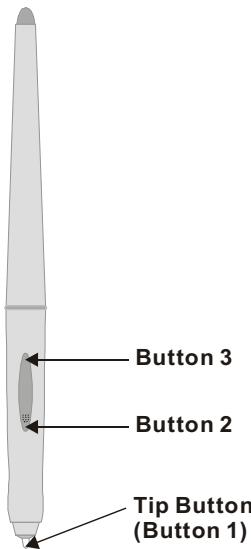
**Button 1** - Also called "Tip Button". This button works like Mouse's left button. It is not programable.
