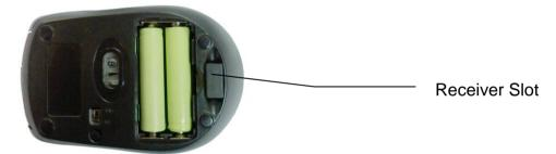
3. Replace the Battery Compartment Cover back onto your Mouse until it securely locks.
