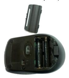
2. Install two AAA Batteries into your Mouse following the battery orientation guide in the battery bay.
