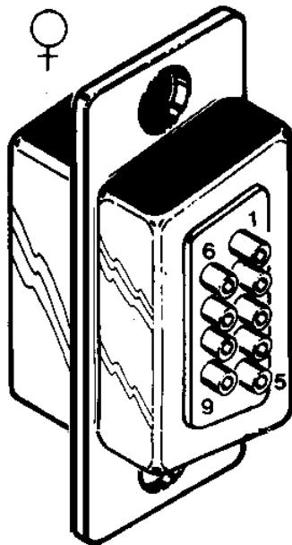
**9-pin sub-D DTE**
