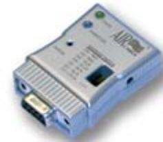
AIRcable modules are intelligent and run firmware-based onboard Bluetooth connection software. There is no need to install and configure extra software to establish a wireless connection. Because the AIRcable is designed to replace physical connections, you can run the same software that would support a physical cable.
