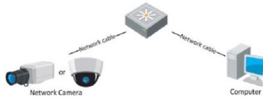
Figure 3-2 Connecting via a Switch or a Router
