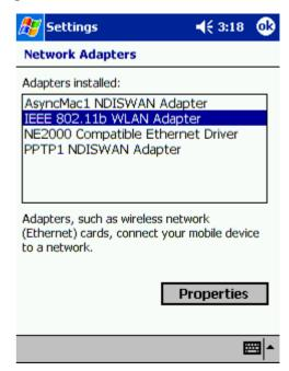
3. Click <u>Start→Programs→IEEE 802.11b WLAN</u>, to view or adjust other configuration settings, such as Mode and SSID etc. Click Apply and Ok to save and implement the settings.
