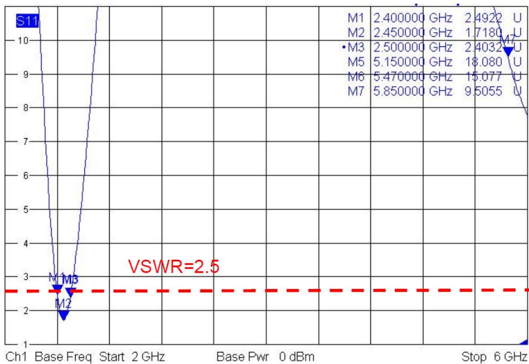
Fig.5 Antenna VSWR (Testing point is same as Fig.6)
