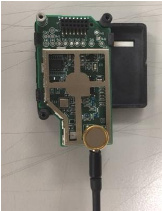
Connection for conducted test
