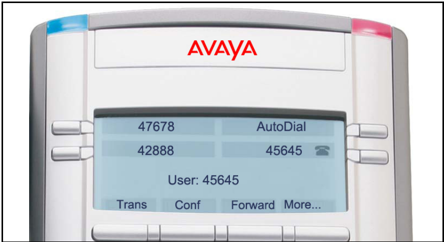
Figure 28: Logged in to an Avaya 1140E IP Deskphone using an Avaya 1120E IP Deskphone
