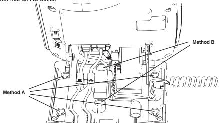
**Step 8: Wall-mount your IP Phone (optional).** Your IP Phone 1165E can be mounted either by: (Method A) using the mounting holes on the bottom of the phone stand, or (Method B) using a traditional-style wall-mount box with RJ-45 connector and 15-cm (6-inch) RJ-45 cord (not provided).
