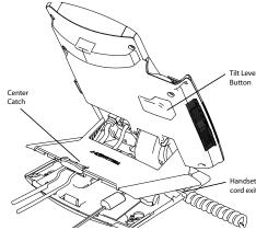
**Step 2: Connect the AC power adapter (optional).** Connect the adapter to the AC adapter jack in the bottom of the phone. Form a small bend in the cable, and then thread the adapter cord through the channels in the stand.
