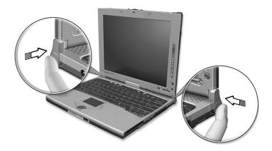
**3** Rotate the display screen 180 degrees clockwise as shown in the illustration. Make sure that the display screen is aligned with the screen supports that will hold it in place.
