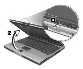
4 Slide the power switch, located on the right panel, towards the rear of the computer (a) then release it (b) to turn on the power. The POST (power-on self-test) routine executes and Windows begins loading.
