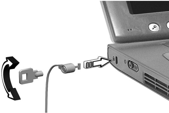
Wrap a computer security lock cable around an immovable object such as a table or locked drawer handle. Insert the lock into the notch and turn the key to secure the lock. Some keyless models are also available.
