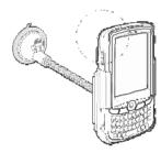
5 Connect the charger cable to the device and connect the other end of the charger cable to the cigarette lighter socket.
