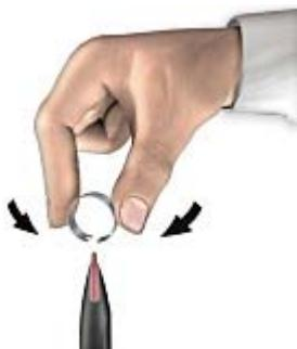
2. Insert a replacement pen tip fully into the Tablet Digitizer Pen.
