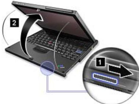
2. Open the display by at least 45 degrees, preferably by 90 degrees. Grasp the center of one side of the computer display with one hand while holding the keyboard bezel with the other hand; then rotate the display slowly clockwise until the back of the display is facing the keyboard. Your computer is now in the **picture frame mode**.
