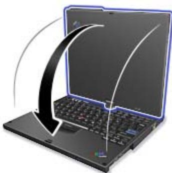
4. Press the center latch down to lock the display.
