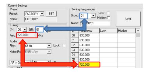
Using the LOAD/SAVE button, at the bottom of the panel, it is possible to **load/save** the frequencies for the selected group from/to a .wdf file. To save the frequencies of all the groups click to the related button above. The legacy option save the channels without the hidden/lock info.
