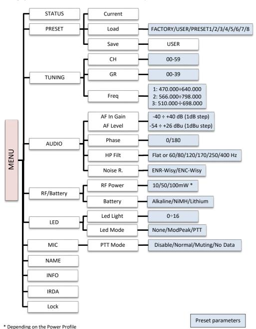
Using <up/down> selector all menus can be accessed in sequence, push <click> to enter edit mode (on the left side of the display appear "EDIT" and the selected parameter starts blinking):
