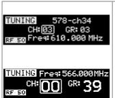
In this menu current channel/group and frequencies can be setup. The name of the group is shown on the top right of the display. Sync group is a quick self-settable channel synchronized by receiver (with SYNC group, on the top right of the display is shown the name of the synchronized receiver).
