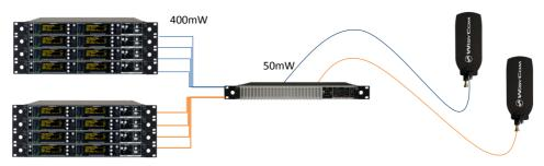
Example2: Combiner [16:1] configuration with high power transmitters:
