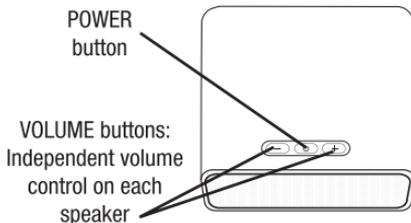
2. For your convenience, the speakers will charge in the recharging cradle, even if the **power** button is turned off. The charging base only needs to be plugged in for the speakers to charge.
