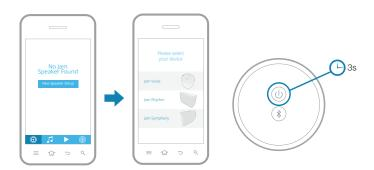
Ensure your device is connected to a wireless network, then open the JAM Wifi app. On the home screen, press New Speaker Setup to connect the speaker. You will be prompted to choose your speaker. Choose "JAM Voice" from the speaker list.
