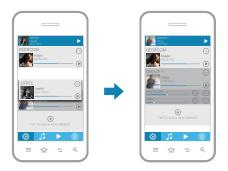
Within the app, press and hold the speaker you would like to group. Drag and drop to pair it with another speaker or add it to an existing group of speakers. The speaker that you are dropping into (or the first speaker listed in a group) is the master speaker.
