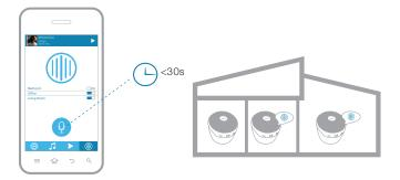
Press the (11) icon within the app, then use the toggle buttons to select the speaker(s) you'd like to broadcast to. Press and hold the microphone icon while saying your message (up to 30 seconds).
