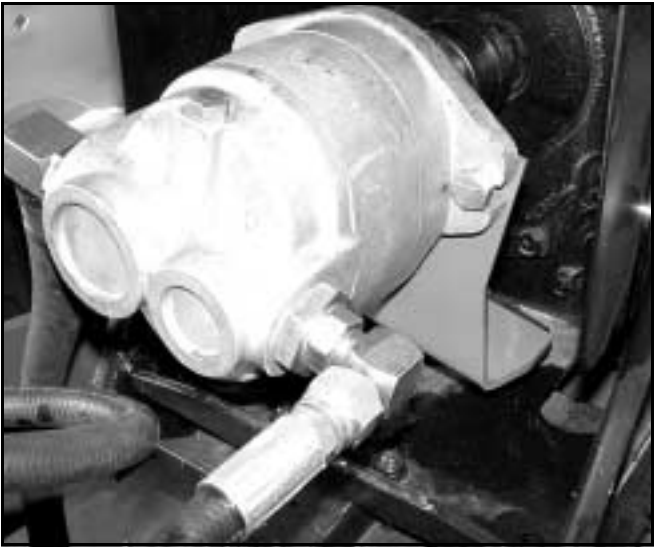
Figure 12 Pump and Bracket Installed
