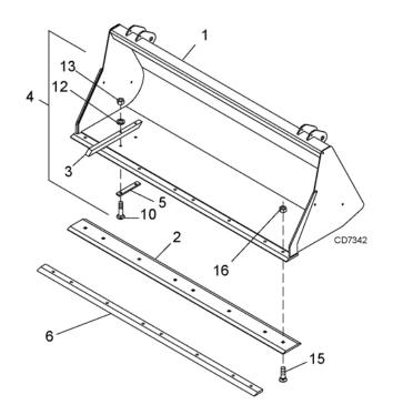
**NOTE**: Bolt-on cutting edge kits and bucket tooth kits are optional and must be ordered separately.
