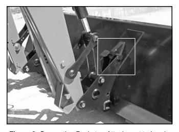
Figure 2. Connecting Bucket or Attachment to Loader
