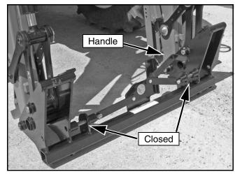
Figure 3. Attachment Coupler Handle - Locked
