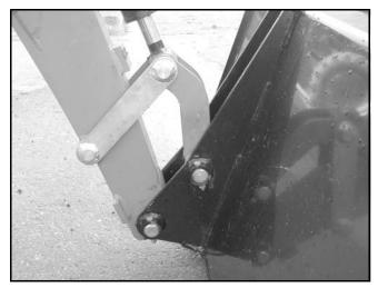
Figure 37. Pin On Bucket Installed (Typical)
