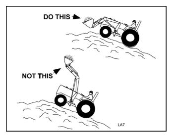
Figure 9. Operating on a Slope
