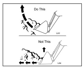
Figure 6. Lift and Rollback Bucket
