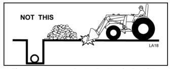
Figure 22. Incorrect Bucket Position for Backfilling
