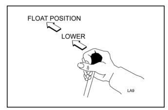
Figure 11. Control Handle Function
