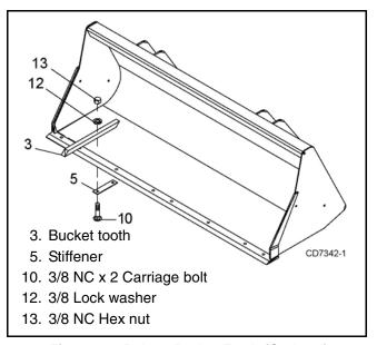
Figure 43. Bolt on Bucket Tooth (Optional)
