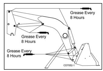
Figure 30. Lubrication Points
