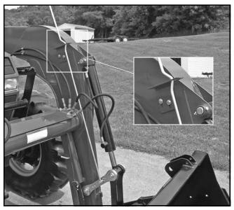
Figure 40. Bucket Level Indicator Installed
