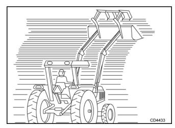
**Figure 27**. Removing Hay and Silage from a Pile with a Grapple Fork
