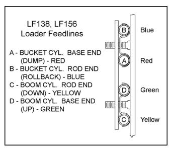
Figure 47. Loader Supply Hose Connection
