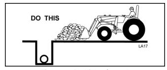
Figure 21. Backfilling Correctly
