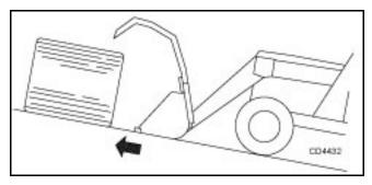
Figure 25. Picking Up Round Bale on a Slope
