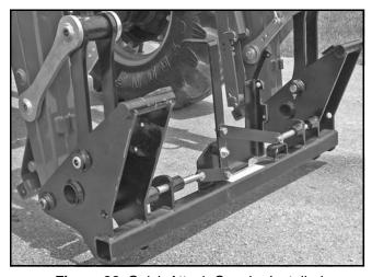
Figure 38. Quick Attach Coupler Installed
