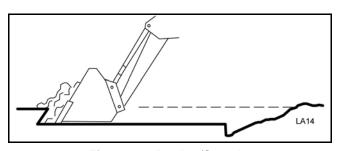
Figure 15. Peeling/Scraping
