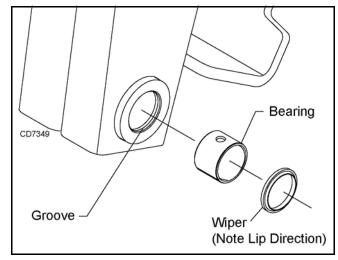
Figure 36. Wiper Installation
