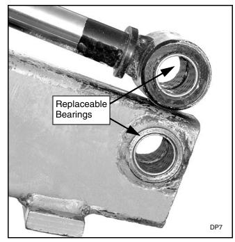
Figure 35. Replaceable Bearings (Typical)
