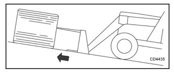
Figure 29. Picking Up Round Bale on a Slope
