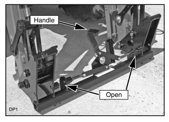
Figure 1. Quick Attach Coupler Handle - Unlocked
