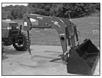
Figure 44. Align Tractor to Loader
