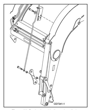
Figure 39. Bucket Level Indicator Installation
