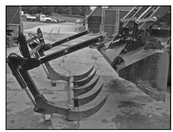
Figure 50. Align Bucket with Grapple
