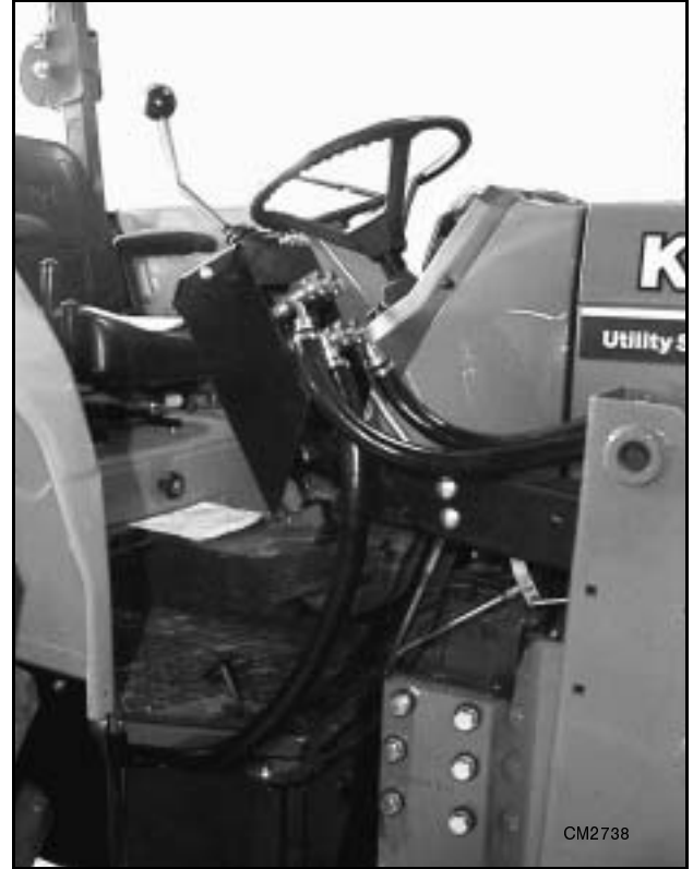
Figure 16 #56037 Control Valve Installed (Typical installation)
