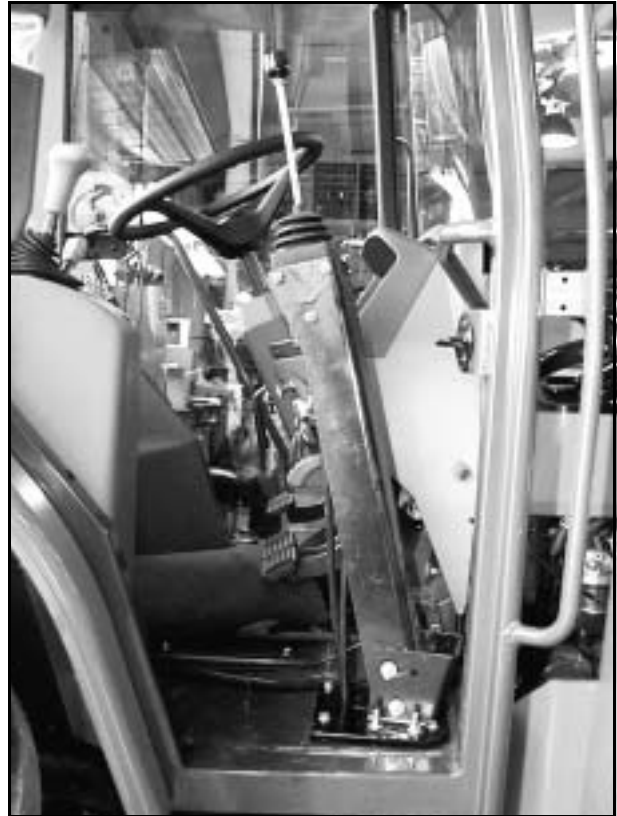
Figure 28 Controller Stand Installed
