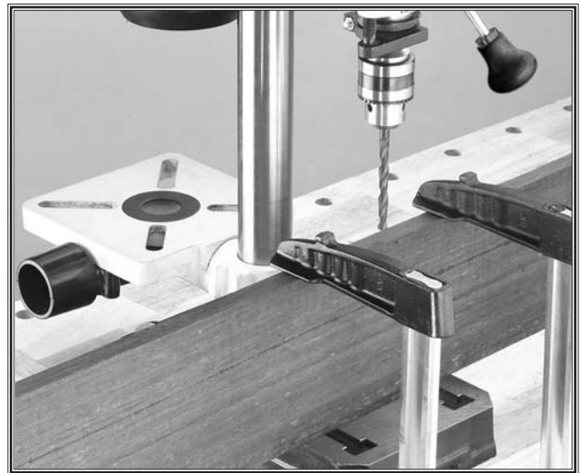
Figure 25. Table adjusted behind column.
