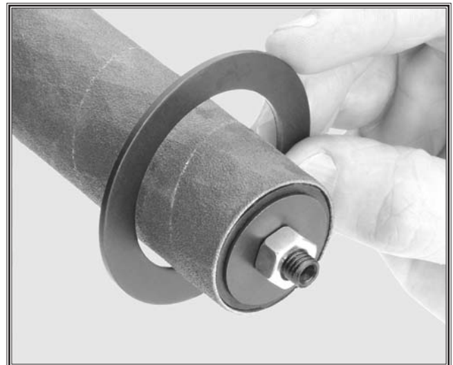
Figure 35. Sanding drum table insert.
