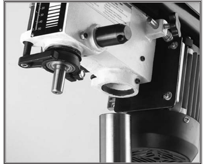
Figure 10. Aligning the pocket in the headstock with the column.
