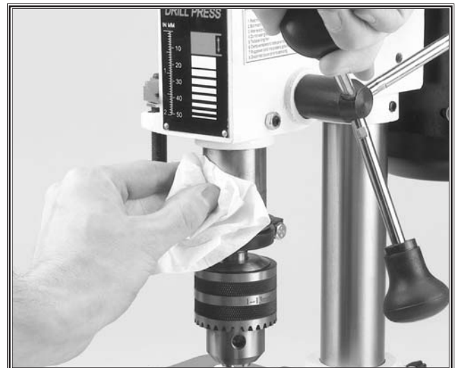
Figure 22. Clean and oil quill shaft.
