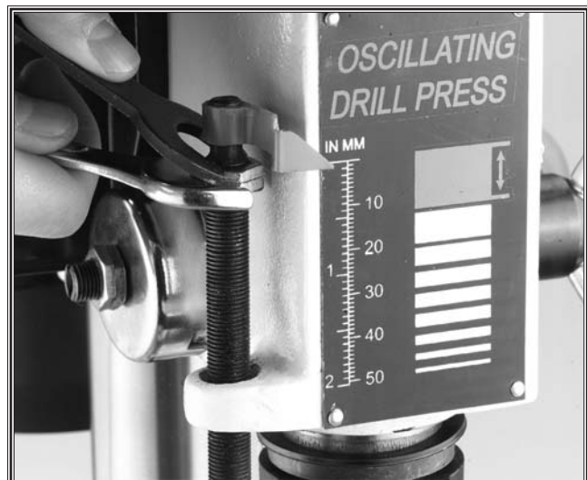
Figure 38. Back-off the depth stop nuts.
