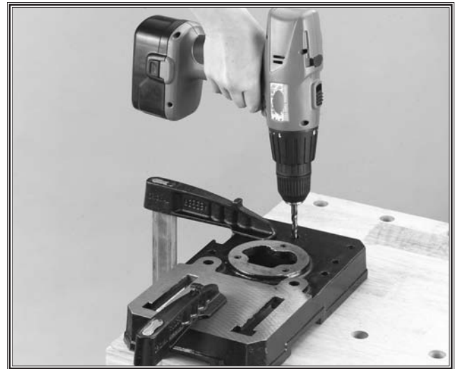
Figure 7. Using holes as a drill guide.
