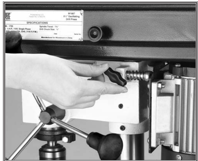
Figure 27. Loosening the lock knob.
