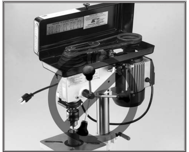
Figure 4. Remove handles when using the oscillating sanding feature.
