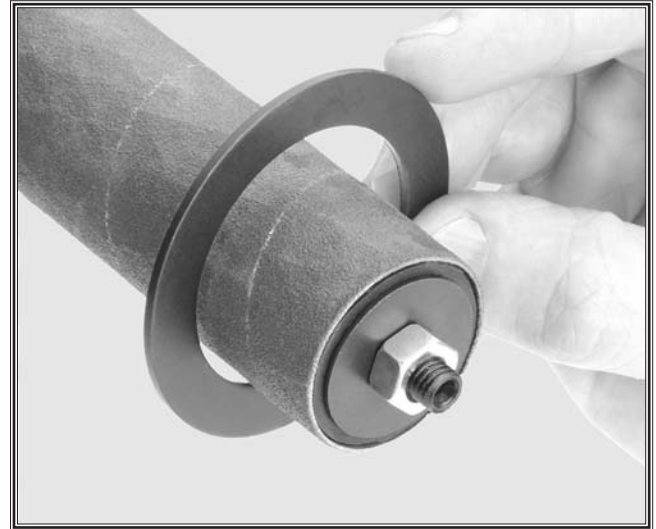
Figure 39. Sanding drum table insert.
