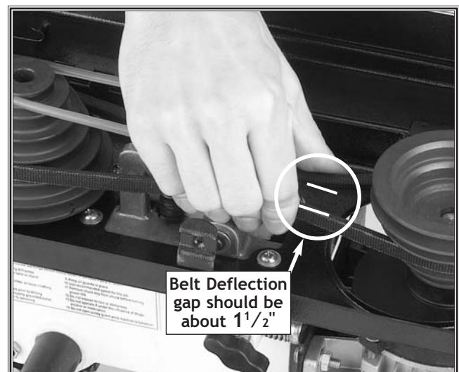
Figure 17. Measuring belt deflection.
