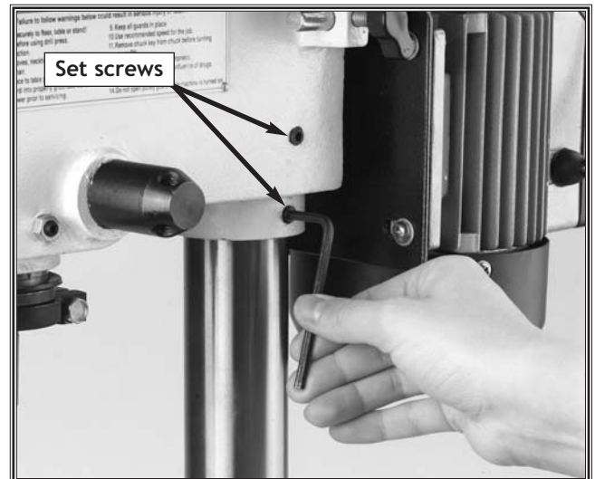
Figure 11. Securing the headstock to the column.
