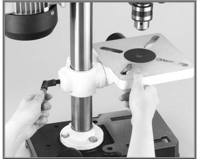
Figure 24. Support table while loosening lock.
