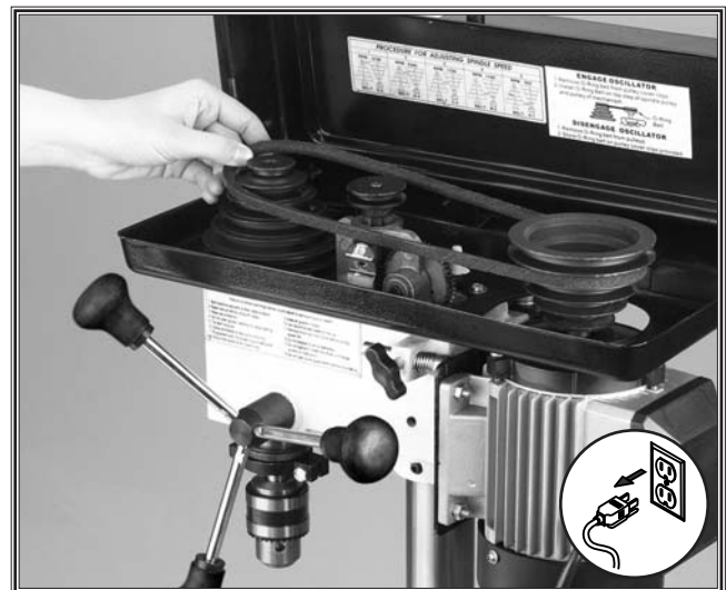
Figure 28. Adjusting belt to desired speed.
