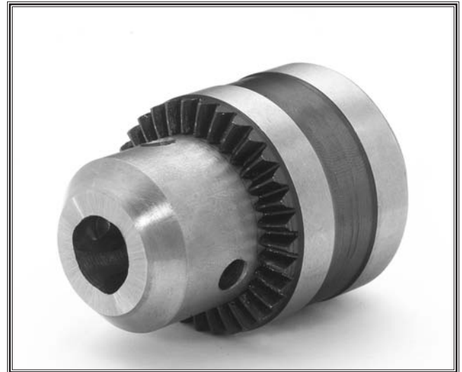
Figure 12. Jaws adjusted inside chuck body.
