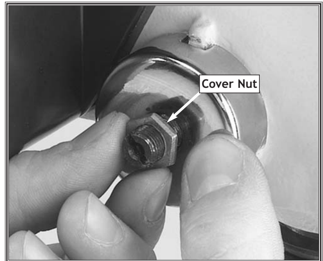
Figure 21. Hold the spring cover tightly.
