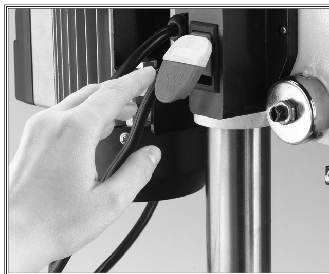
Figure 39. Hand poised over a typical stop switch.
