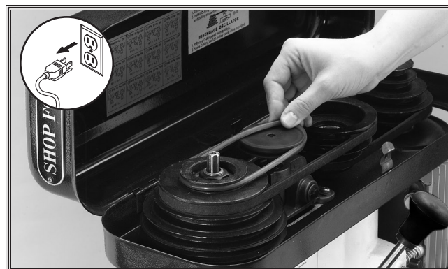
Figure 44. Stretch the belt to fit on pulleys.
