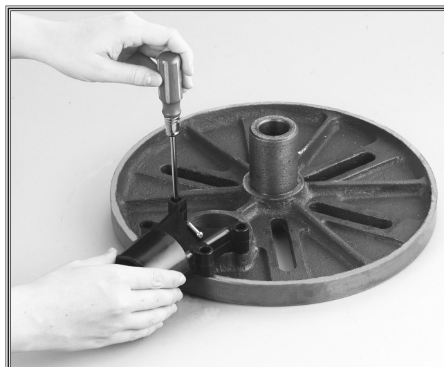
Figure 9. Installing the dust port.
