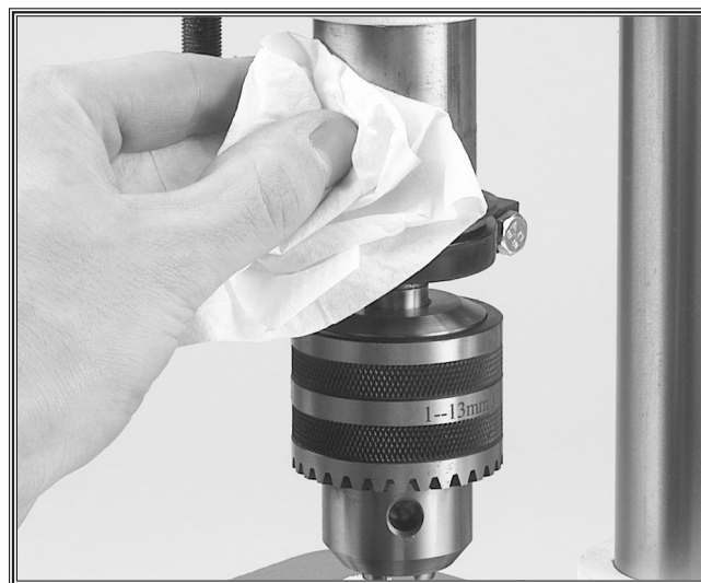
Figure 28. Clean and oil quill shaft.
