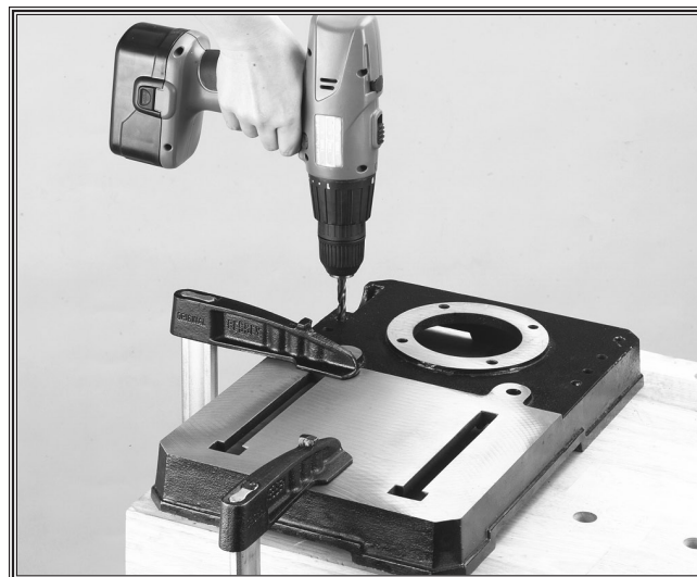
Figure 8. Using holes as a drill guide.
