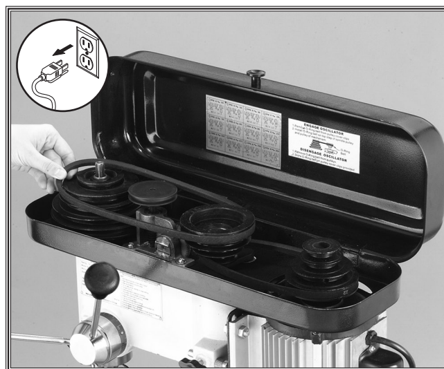
Figure 34. Adjusting belt to desired speed.
