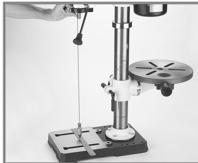
Figure 17. Aligning headstock with base.
