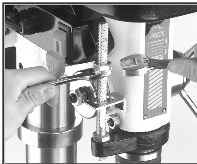
Figure 45. Back-off the depth stop nuts.
