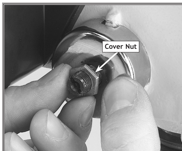
Figure 27. Hold the spring cover tightly.
