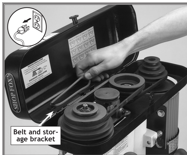
Figure 43. Oscillator belt on storage bracket.
