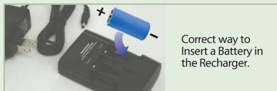
Correct way to Insert a Battery in the Recharger.
