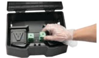
7. Upon closing the lid, a green LED on the top of the box will start blinking and will begin to blink faster as calibration progresses. When complete, the green LED will turn off and your bait box will be ready.
