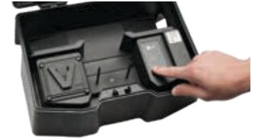
5. Upon closing the lid, a yellow LED on the top of the box will start blinking and will begin to blink faster as calibration progresses. When complete, the yellow LED will turn off and a green LED will turn on.
