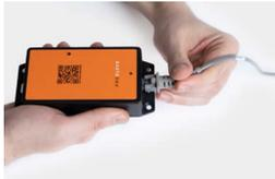
2. Plug the other end of the USB cable into the RJ45 socket of the Access Point One S. A clear clicking sound confirms the correct fastening.
