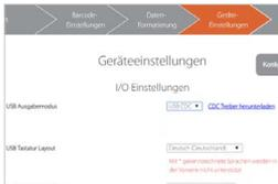
3. In the configuration tool ([config.proglove.de](http://config.proglove.de)) under "Device settings - USB output mode," select USB CDC. [More detailed information about this can be found in chapter 5 "Configuration tool."](#)
