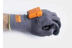
1. Press the textile trigger on the glove in order to activate the crosshairs.
