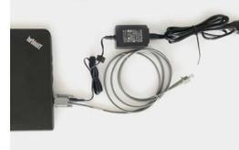
1. Connect the RS232 with the end device. Connect the power supply to the RS232 and into an external power source.
