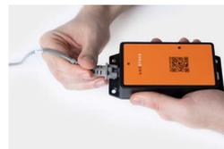
2. Once the safety closure has been pressed, disconnect the connection cable out of the RJ45 socket.
