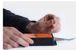
1. Press an elongated object (e.g. paper clip) into the opening on the top of the Access Point One S to open the safety closure.
