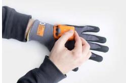
1. Position MARK 2 on the fastening rail of the glove. The pins face down.
