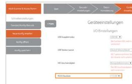
3. Check which baud rate must be set. The baud rate is set to 115,200 as a standard. At a different baud rate, this is to be set in the configuration tool ([config.proglove.de](http://config.proglove.de)). [More detailed information about this can be found in chapter 5 "Configuration tool."](#)
