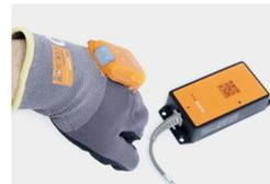
2. Aim MARK 2 crosshairs on the Access Point One S and scan the pairing barcode.
