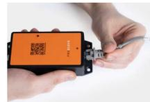
2. Plug the other end of the USB cable into the RJ45 socket of the Access Point One S.
