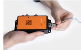
2. Plug the other end of the cable into the RJ45 socket of the Access Point One S. A clear clicking sound confirms the correct fastening.
