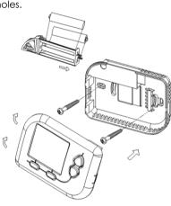
Insert two fresh AAA alkaline batteries into the drawer according to the polarity marked inside, then slide the drawer back into the place as shown in the above Figure.
