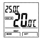
When user enter setting mode, room unit display SETTING icon. The top left corner value will be room temperature.
