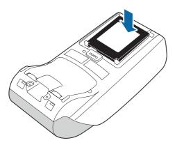
Figure 15. Clicking battery in place
