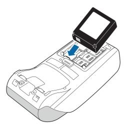
Figure 14. Inserting the battery
