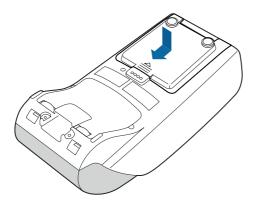
Figure 16. Closing the battery cover
