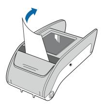
Figure 13. Tearing off paper
