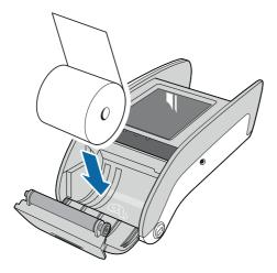
Figure 11. Inserting paper roll
