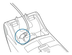
Figure 19. Power input socket underneath terminal
