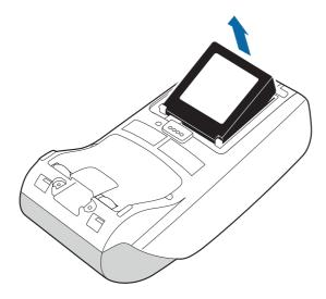
Figure 26. Removing the battery
