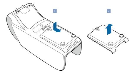
Figure 25. Removing card/battery cover
