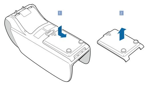
Figure 7. Removing the card/battery cover
