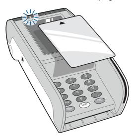
Figure 23. Reading a smart card with the contactless reader
