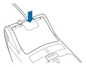
Figure 20. Closing the connector compartment
