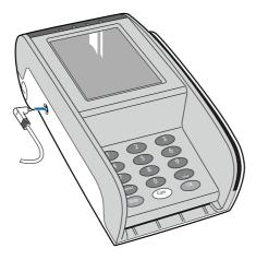
Figure 17. Connecting the battery charger
