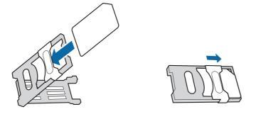
Figure 9. Inserting card and closing holder
