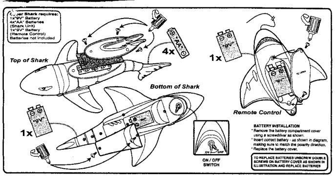
CAUTION: After each use of the Cyber Shark remove all batteries from the product, and drain any water that has accumulated inside. Moisture allowed to remain inside the product will damage the electronic components and batteries. Store the product with the battery compartment door open to allow the compartment to dry completely.
