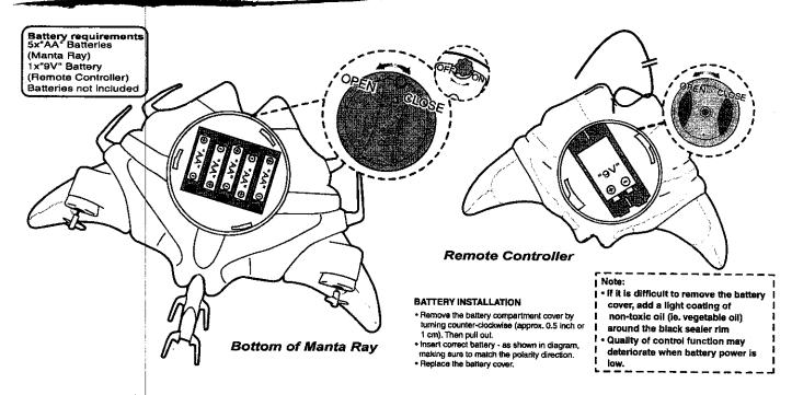
**CAUTION:** After each use of Manta Ray remove all batteries from the product, and drain any water that has accumulated inside. Moisture allowed to remain inside the product will damage the electronic components and batteries. Store the product with the battery compartment door open to allow the compartment to dry completely.
