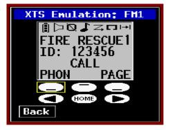
The XTS-Emulation page will show what the internal transceiver normally would show on its screen. The 6 soft keys on the handheld are accessed using virtual buttons selectable via the Select Knob. Pressing ENTER while one of these keys is selected shall send the appropriate "key pressed" message to the radio. Pressing any of the keypad keys sends the appropriate "key pressed" message to the radio. Pressing ENTER while the "BACK" button is selected returns the operator to the previous screen.
