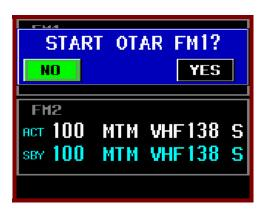
• To confirm the start of the OTAR, select YES and press the ENTER button to initiate the OTAR process. The status of the OTAR will be displayed on the radio's display line. Status messages include "OTAR REQUESTED", "OTAR IN PROGRESS", "OTAR ABORTING", "OTAR COMPLETE", and "OTAR FAILED".
