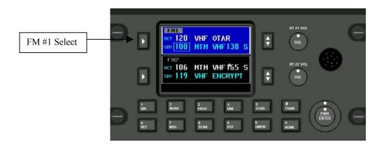
To make FM1 the active transceiver: Push the FM #1 SELECT BUTTON (shown above). Pushing the FM #2 SELECT BUTTON will make FM2 the active transceiver and the blue highlight will be moved to the FM2 area of the display (shown below).
