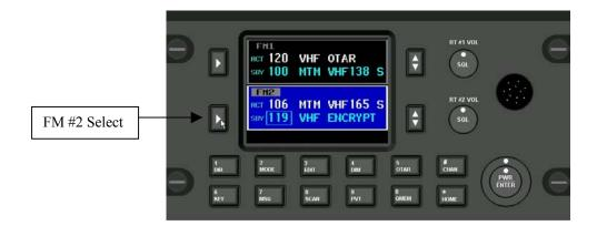
When the P-2000 operating in MODE 1 (only one headset shared between two transceivers), the active transceiver is the one that will be used for transmitting. In MODE 1, the transceivers (FM1 and FM2) will have their receive audio summed together and sent to the headset. The operator must choose which transceiver will be used when they want to transmit.
