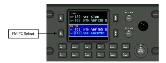
When the P-2000 is operating in SINGLE MIC MODE (only one headset shared between two transceivers), the active transceiver is the one that will be used for transmitting. In Single Mic Mode, the transceivers (FM1 and FM2) will have their receive audio summed together and sent to Headset #1. The operator must choose which transceiver will be used when they want to transmit.
