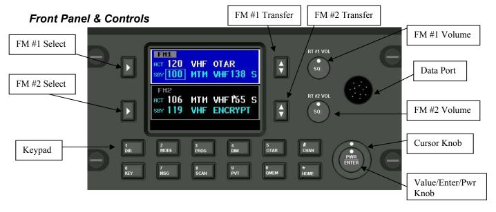
DISPLAY - The P-2000 has a color LCD display. It provides the visual feedback for the system. Exactly what is displayed depends on the current operating mode of the P-2000. During normal operation, the top area shows information for FM #1 and the bottom line shows information for FM #2.
