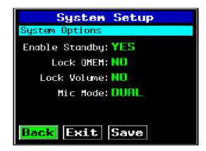
• To Save the changes made to the SYSTEM SETUP, highlight the "SAVE" option and press enter. The screen will indicate saving of the data is taking place. When the data save process is complete, press the HOME button several times until the HOME page is displayed.
