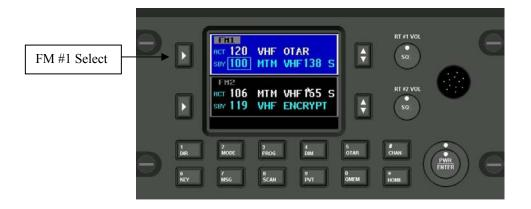
To make FM1 the active transceiver, push the FM #1 SELECT BUTTON as shown above. Pushing the FM #2 select button will make FM2 the active transceiver and the blue highlight will be moved to the FM2 area of the display as shown below.
