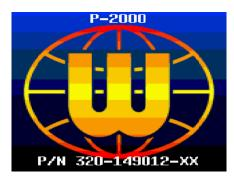
To power the P-2000 OFF, press and hold the PWR button for 3 seconds. The following message flashes on the display several times:
