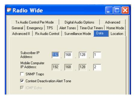
(11) TX Audio Control Per Mode – This menu allows you to chance transmit audio control elements radio wide.
