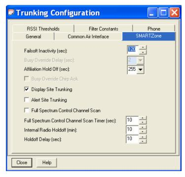
**Note:** Older Archive CPS files contained "Display Site Trunking" ENABLED. However this must be DISABLED in order to function properly with customer trunking systems.
