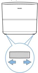
The device compensates for the distortion from the slanted projection (pincushion distortion).
