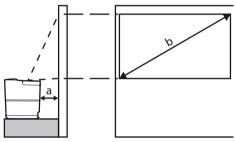
To change the size of the screen, just move the projector towards or away from the wall. The size of the screen (b) is comprised between **0.1 and 0.42** metres depending on the projection distance (a), as described in the following table.
