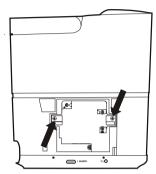
1 Pull out the lamp by inserting your fingers in the two slots
