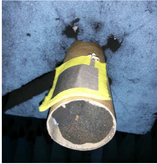
Figure 4.2 - Cloth antenna under test in the chamber
