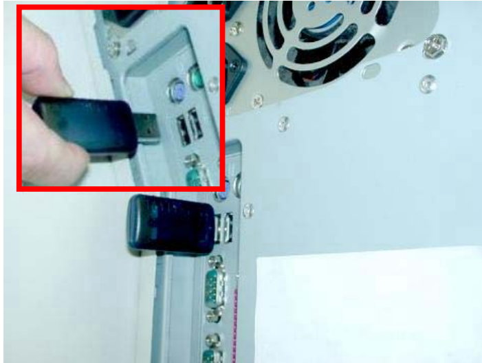
Figure 3-1: Plug the Bluetooth USB Adapter into USB port on desktop PC
