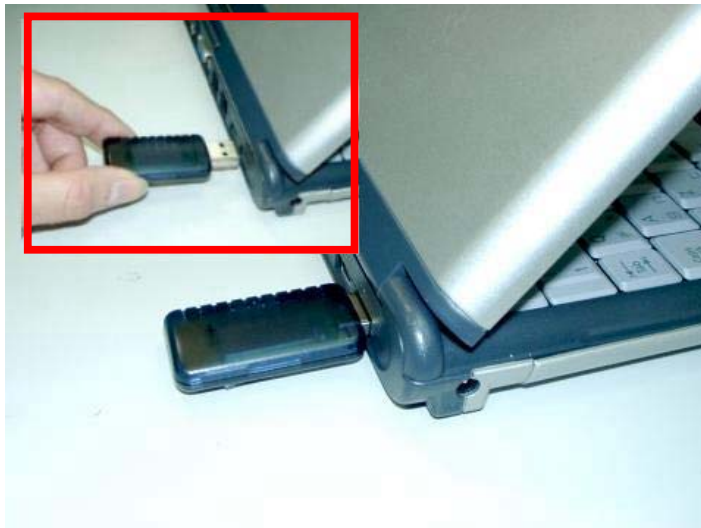
Figure 3-2: Plug the Bluetooth USB Adapter into USB port on laptop PC
