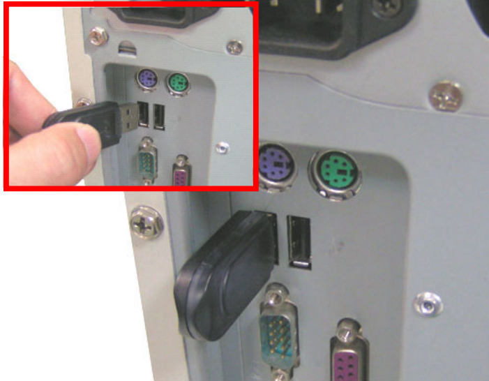
Figure 2-9: Plug the Bluetooth USB Adapter into USB port on desktop PC
