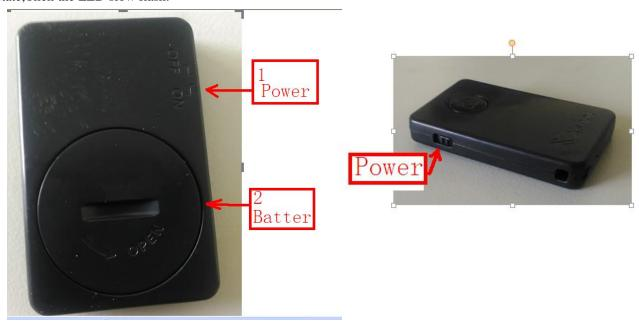
Pictured above, in "OPEN" direction of rotation Battery battery cover, can remove the battery cover to replace the CR2032 battery, replace the installed back battery cover and rotated in reverse direction.
