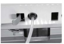
After removing the filament, plug the filament tube directly back to its original position to complete the re-installation.
