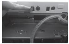
2 If the filament is stuck at the entrance of the guide tube, please press the release arm by the entrance to extract the stuck filament
