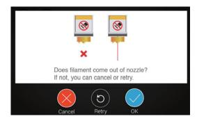
6 If filament doesn't come out from the nozzle, please press "Retry" or "Cancel". When filament is dripping off the nozzle, tap to finish.
