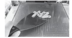
5 Remove the printed object when the print bed has descended.
