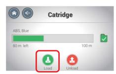
4 Select "Filament" > "Cartridge " > "Load".
