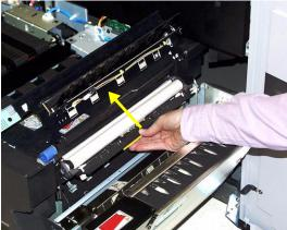
Figure 19. Raise the unit into place
