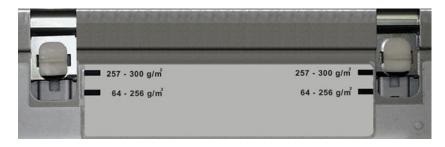
Figure 5. Air Adjustment Levers
