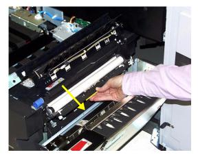
Figure 17. Pull the unit down and out
