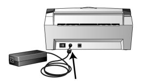
2. Plug the power cord into the power supply and into a wall outlet.
