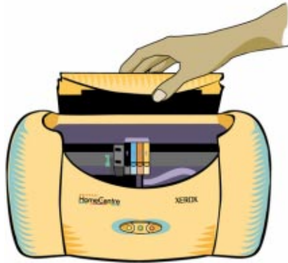
Open cover showing printhead and ink cartridges
