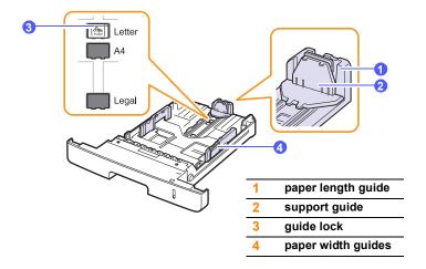
1 Press and hold the guide lock, and slide the paper length guide to locate it in the correct paper size slot.
