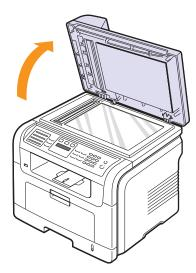
2 Place the original **face down** on the scanner glass and align it with the registration guide at the top left corner of the glass.
