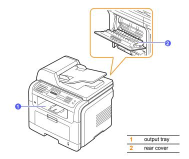
The printer sends output to the output tray by default. To use the output tray, make sure that the rear cover is closed.
