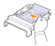
If the paper does not come out with the duplex unit, remove the paper from the bottom of the machine.
