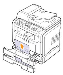
5 Insert the trays back into the machine. Printing automatically resumes.
