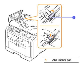
4 Insert a new ADF rubber pad into place.
