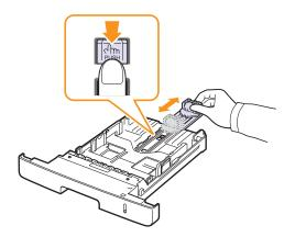
2 After inserting paper into the tray, adjust the support guide so that it lightly touches the paper stack.
