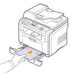
If the paper does not move when you pull, or if you do not see the paper in this area, check the fuser area around the print cartridge. See page 14.3.
