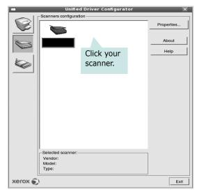
When you have only one MFP device and it is connected to the computer and turned on, your scanner appears on the list and is automatically selected.
