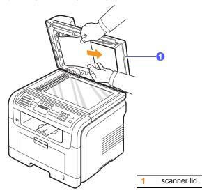
**3** Close the scanner lid. Then load the removed pages back into the ADF.
