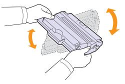
Thoroughly roll the cartridge to assure maximum copies per cartridge. Save the box and the plastic bag for shipping.
