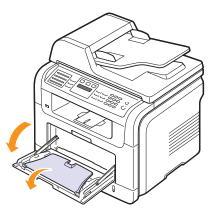
**2** If you are using paper, flex or fan the edge of the paper stack to separate the pages before loading.
