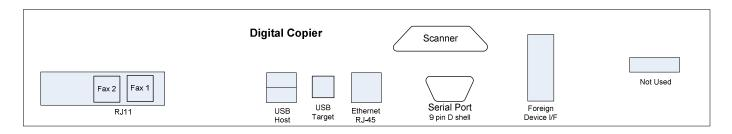
Figure 2-3 Back panel connections
