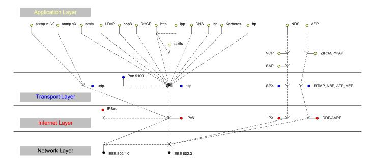
Figure 2-6 IPv6 Network Protocol Stack
