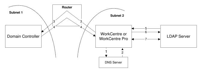
2) The DNS Server returns the IP Address of the Domain Controller
