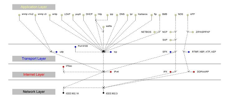
Figure 2-5 IPv4 Network Protocol Stack
