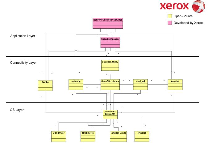
Figure 2-4 Controller Operating System layer components
