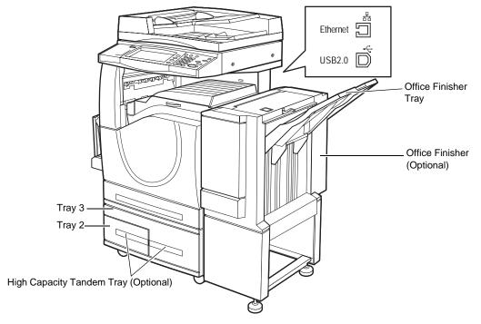
**NOTE:** Depending on the configuration, the Document Glass Cover is attached instead of the Document Feeder. Two optional paper trays can be attached.
