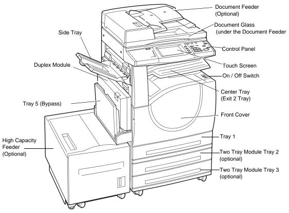
The following diagrams show the standard and optional components of the machine. Configuration may vary depending on the model.
