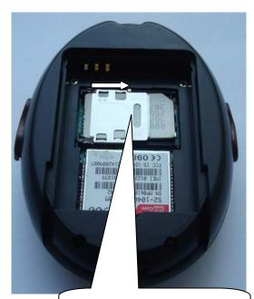
After SD card is mounted, Fasten the simcard rightwards
