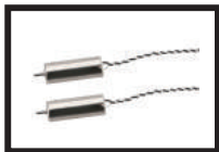
Counterclockwise motor (white/black wire)
