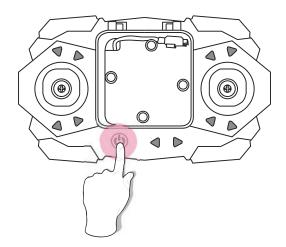
③ Then, trun on the Transmitter. One second later, one beep will be heard and the drone's indicator lights will start flashing and then turn solid, indicating that the drone and the transmitter have been paired successfully and automatically.
