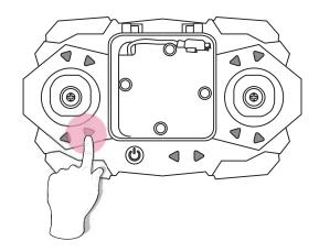
**6** Press One Key Take-off button, the drone will take off automatically. Or push throttle(left) joystick up slowly to take off and ascend the drone.
