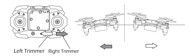
**9 Left/ Right Sideward Fly Trim:** When the drone drifts to left, press the right trimmer button to rebalance the drone; if the drone drifts to right, press the left trimmer button to reblance the drone.
