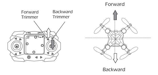
**10** Forward/ Backward Sideward Fly Trim: When the drone drifts forward, press the backward trimmer button to rebalance the drone; if the drone drifts backward, press the forward trimmer button to rebalance the drone.
