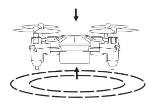
During flight, altitude hold function allows you to release the throttle joystick, and the drone will keep hovering at the current height.
