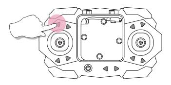
This drone comes with 3 speed modes (Low/ Medium/ High). Press the "Speed Switch" button on transmitter to switch the speed mode. "Di" from the transmitter indicates it is in low speed mode, "DiDi" indicate medium speed, and "DiDiDi" indicate high speed. (Low speed will be default mode!)
