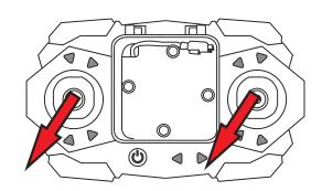
Pull both joysticks down to the bottom left at the same time, then the drone's lights will blink and turn solid, indicating the drone's trimmer data is reset (This step can only be done before the drone take off).
