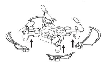
Install the propeller guards to motor base.
