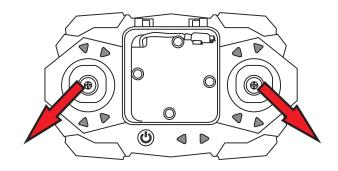
⑤ After pairing or calibration, pull left joystick down to the bottom left, the right joystick down to the bottom right at the same time. The LED indicator lights on the drone will blinking and turn sold again, and the propellers will start spinning, indicating that the drone is unlocked and ready to take off.
