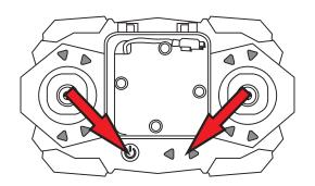
④ After pairing, push the left joystick down to the bottom right and the right joystick down to the bottom left at the same time. A beep sound will be heard from the transmitter and the LED lights of the drone will blinking, then turn solid, indicating that the calibration setting is completed.
